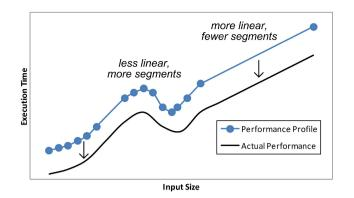
Figure 1. A comparison of actual implementation performance and the performance profile output of the planner (*shifted up for visualization*), which determines maximum-sized regions that can be linearly approximated.
