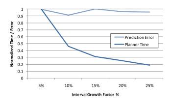
Figure 9. Effect of changing the interval growth factor on planner time and prediction error.
