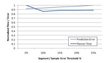
Figure 10. Effect of changing the segment error threshold and sample error threshold (both set to the same value) on planner time and prediction error.
