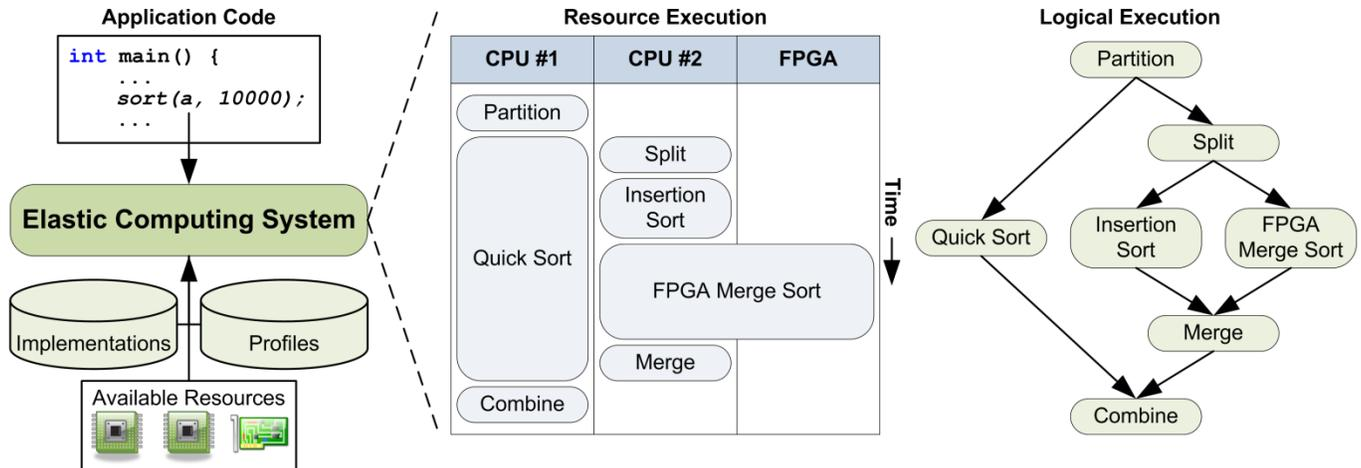
**Figure 5.** When an application executes an elastic function, the *elastic computing system* uses the performance profiles from implementation planning to select and execute the fastest implementation for the available resources and input parameters.
