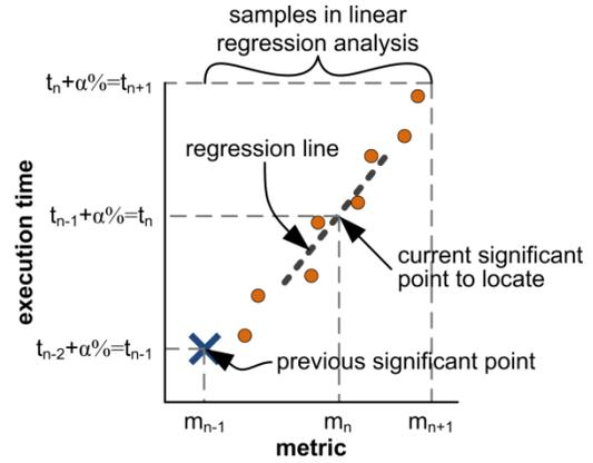
Figure 4. Illustration of performance profile generation.
