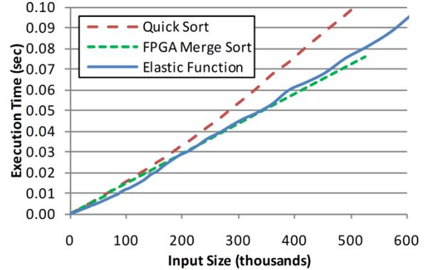
**Figure 8.** Elastic computing adaptability for a hyper-threaded Intel Xeon system with a Nallatech H101-PCIXM FPGA accelerator, showing that for all input sizes, elastic computing achieves the best (or near best) implementation.
