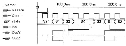
(a) Construct an ASM diagram that will produce the above behavior.
