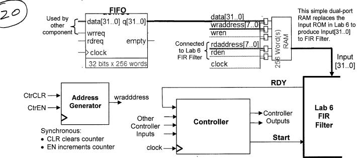
You are to design the <u>controller</u> of following component to fill the Input RAM for a Lab 6 FIR filter (from Location 0 to Location 256). Note that the Input RAM plays the same role as the Input ROM in Lab 6.
