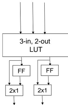
Map the following circuit onto these CLBs by drawing boxes to represent CLBs. **Do not try to optimize or modify the circuit in any way.**
