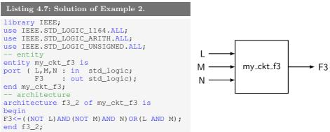
This example shows a one-line implementation of the given logic equation.
