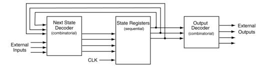
Figure 7.1: Block diagram for a Moore-type FSM.
