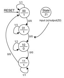
**SOLUTION.** The state diagram indicates that its implementation will contain four states, one external input and two external outputs. This is a hybrid FSM in that the if contains both a Mealy and Moore-type output but in this case, the FSM would be considered a Mealy-type FSM. The black-box diagram and the actual solution for the solution is shown in listing 7.4.
