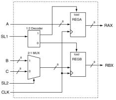
**EXERCISE 6.** Provide a VHDL model that can be used to implement the following circuit.
