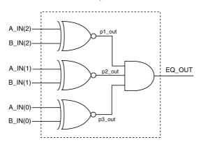
Figure 8.1: Discrete gate implementation of a 3-bit comparator.
