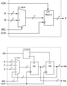
**EXERCISE 3.** Provide a VHDL model that can be used to implement the following circuit.
