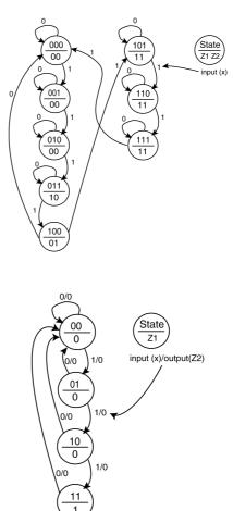
**EXERCISE 9.** Write the VHDL behavioral model code that can be used to implement the state diagram shown on the right. The state variables should be encoded as listed and also provided as outputs of the FSM.
