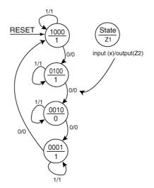
**SOLUTION.** The state diagram shows four states, one external input X, two external outputs Z1 and Z2 with the Z2 output being a Mealy output. This is a Mealy machine that indicates one-hot encoding should be used to encode the state variables. We will approach the implementation of this FSM one piece at the time.
