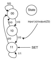
**SOLUTION.** The state diagram shown in this problem indicates that this is a threestate FSM with one Mealy-type external output and one external input. Since there are three states, the solution requires at least two state variables to handle the three states. The black-box diagram of the solution is shown in listing 7.3. Note that the two state variables are handled as a bundled signal.
