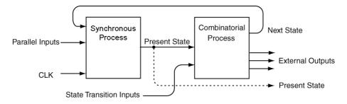
Figure 7.2: Model for VHDL implementations of FSMs.
