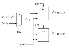
**SOLUTION.** The circuit shown in Example 24 includes two 8-bit registers and a 2:1 MUX. This is an example of a bus-based data transfer in the output of the MUX that is connected to the inputs of the two registers. Each of the two registers has its own independent load control input. The solution to Example 24 is shown in listing 9.1. And as we have grown to expect, there are a couple of things worth noting about this solution.
