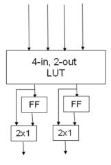
Map the following circuit onto these CLBs by drawing boxes to represent CLBs. Assume that the rectangle components are flip flops and that everything else is combinational logic. Use the minimum number of CLBs for full credit.
