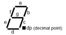
Figure 1. Voltage Table and diagram for the 7 Segment Display
