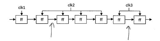
6) (4 points) You are designing a pipelined circuit that requires high bandwidth from an external memory running at a different clock frequency. What synchronizer is most effective for this situation?
