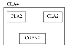
5. Fill in the HIERARCHICAL architecture in adder.vhd with an 8-bit hierarchical CLA using a structural description that connects two of the 4-bit CLAs with one carry generator. This will be very similar to the previous step.
