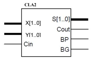
3. Design a carry generator (cgen2.vhd) entity that calculates carries (Ci+1 and Ci+2), block generate (BG), and block propagate (BP) for 2 instances of the 2-bit CLA (see next step for clarification). The lectures notes will describe the exact purpose of this block, but it will be used to hierarchically define CLAs. Use a behavioral architecture. Note that the block propagate and generate are a function of the P and G of each 2-bit CLA, but it is up to you to figure out the exact logic.
