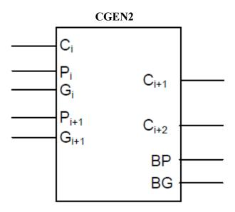
4. Create a 4-bit hierarchical CLA (cla4.vhd) entity with a structural architecture that connects 2 of the 2-bit CLAs with one of the carry generators. It is up to you to determine the exact connections. See lecture notes and section 5.4.
