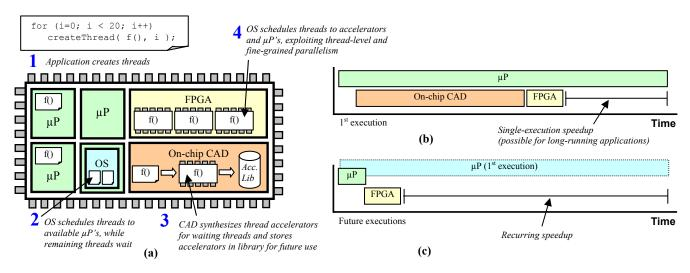
**Figure 1:** Thread warping: (a) architecture and overview, (b) usage when application runtimes greatly exceed synthesis times, as for scientific computations that run for hours or days, (c) usage when applications repeat, in which case synthesized results can be stored in a library and retrieved when needed.
