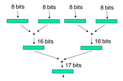
As shown, the datapath has 4 8-bit inputs which connect to two multipliers followed by an adder. The green boxes are all registers of the specified widths. You can create the datapath entity however you want, but it must synthesize to the exact structure shown. The multipliers should generate a 16-bit output and the adder should produce a 17-bit output to prevent overflow.
