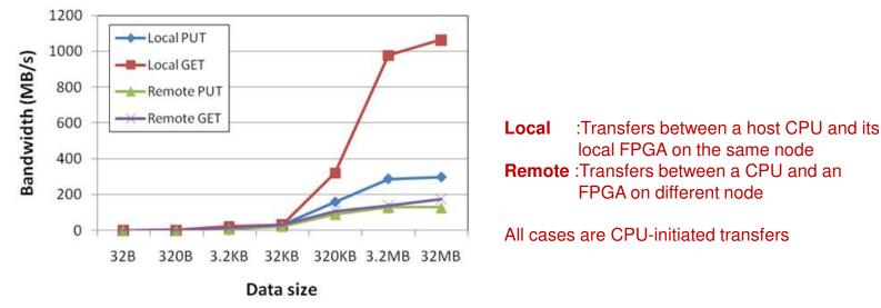
Transfers between CPU and FPGA
