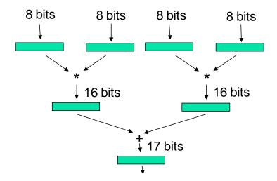
As shown, the datapath has 4 8-bit inputs which connect to two multipliers followed by an adder. The green boxes are all registers of the specified widths. You can create the datapath entity however you want, but it must synthesize to the exact structure shown. Therefore, I would recommend a structural description of registers, multipliers, and an adder. The multipliers should generate a 16-bit output and the adder should produce a 17-bit output to prevent overflow.
