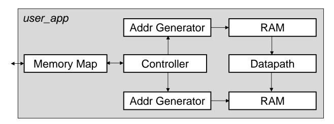
The overall structure of the circuit is shown above. You will use a memory map similar to the previous lab. However, for this lab, the memory map also handles transferring data to and from block RAMs. This code is already provided for you. However, you must create all other components.
