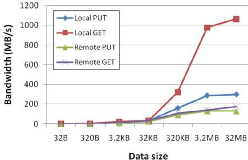
**Local** : Transfers between a host CPU and its local FPGA on the same node
