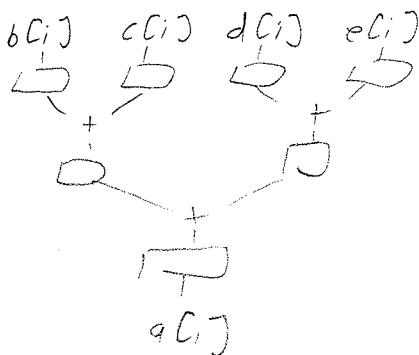
The pipeline would likely stall because the 4 arrays may be stored in different parts of memory.
