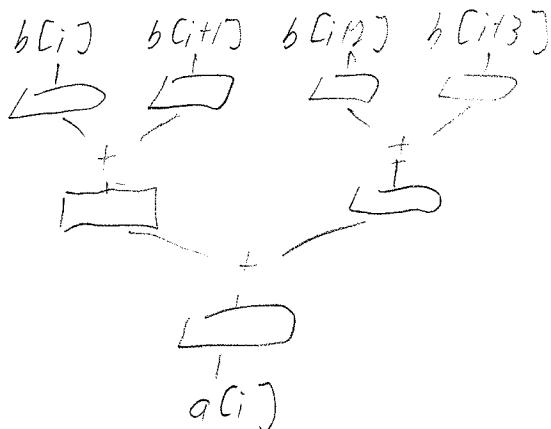
For unrolling to not cause stalls, circuit requires 4 inputs each cycle
