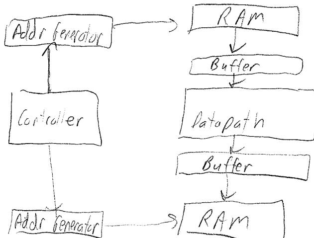
2. Create a fully-pipelined datapath for the following code. Do not unroll the loop.
